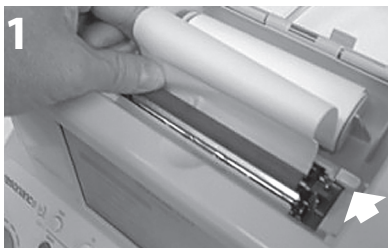
Lever printer locked in print position (down).
